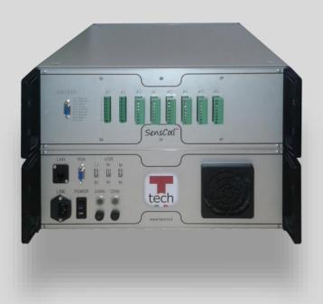
SensCal<sup>m</sup> is a tester specifically designed for the mass production of angular position sensors, as widely used in throttle bodies, variable nozzle turbocharger, 3-way valves and more.
