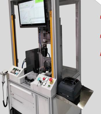
HT-EOL<sup>™</sup> is a stand-alone machine designed for test of electric hand throttles. It can handle resistive (potentiometric) sensor and hall-effect sensor.
