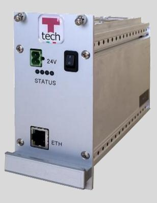
ALL.Pg compact industrial solution for programming the Allegro magneto-resistive sensors of A1340 series.
